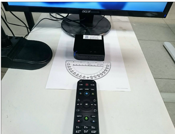
Setup for horizontal test (Desk lamp off)
